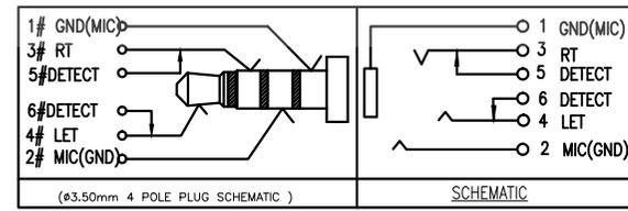
(ø3.50mm 4 POLE PLUG SCHEMATIC )
