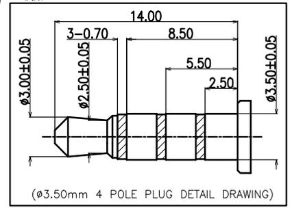
(ø3.50mm 4 POLE PLUG DETAIL DRAWING)
